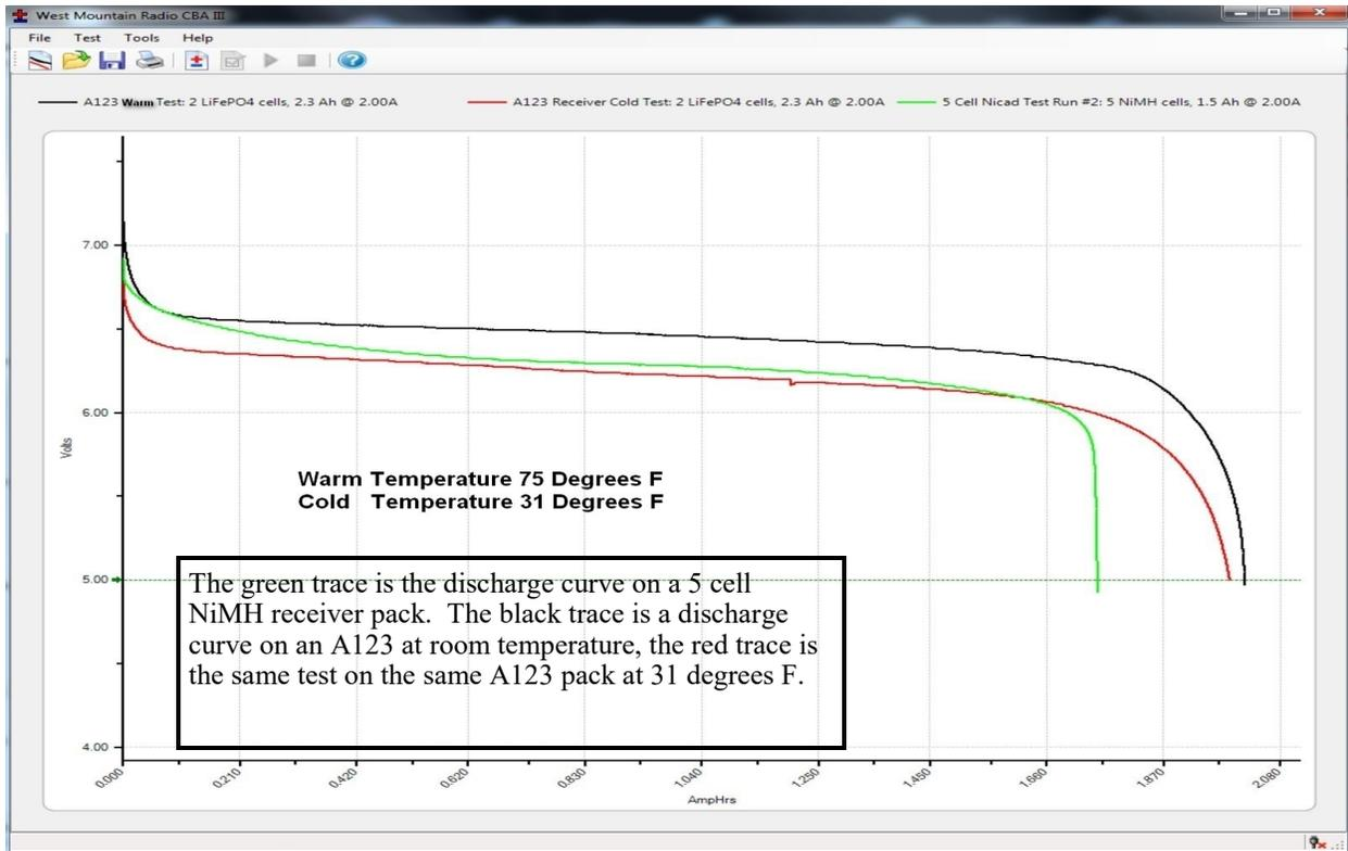
— 5 Cell Nih test 14 Amps: 5 NiMH cells, 1.0 Ah @ 14.00A (0.00 Ah, 0.3%) — 6 Year Old two cell A123 Pack: 2 LiFePO4 cells, 2.3 Ah @ 14.00A
